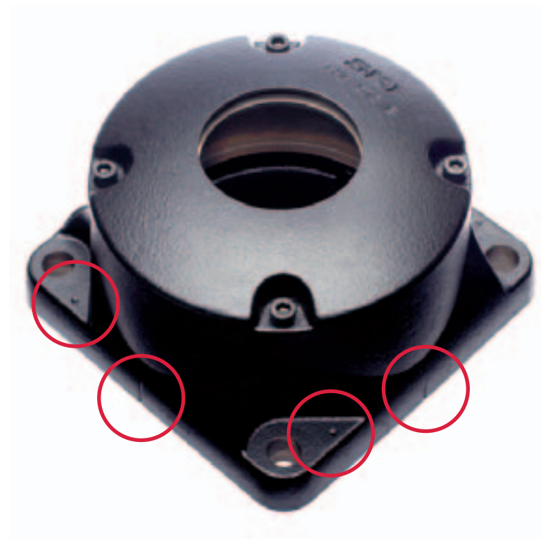
Alignment is made easier by clear marks on the bearing seating centre and drilling position dimples for dowel pins.
